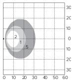
Footcandle calculations based on standard building reflectance of .10 with a ground reflectance of .0 and a light loss factor of .90.
